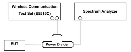
(Configuration of conducted Emission measurement) Test Procedure
