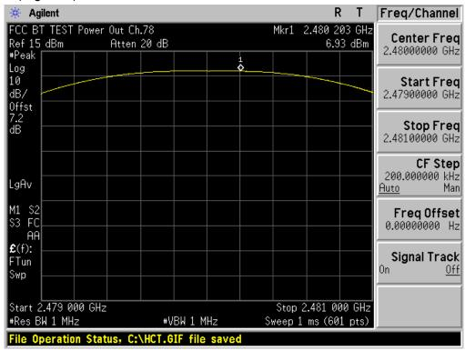
Test Plots (8DPSK) Peak Power (Low-CH)
