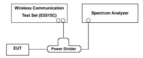
(Configuration of conducted Emission measurement)
