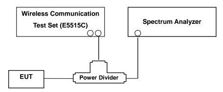
(Configuration of conducted Emission measurement) Test Procedure
