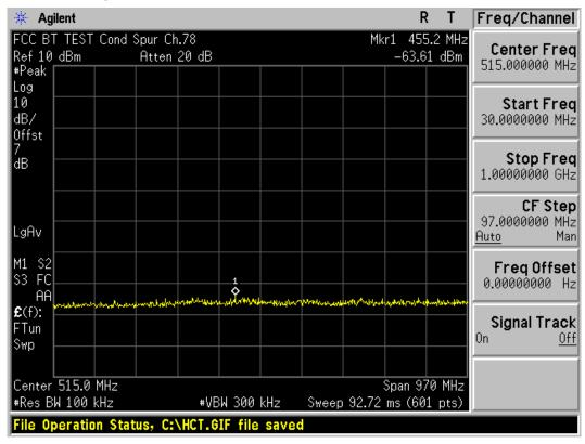
Test Plots (8DPSK) - 30 MHz - 1 GHz (RBW:100 kHz, VBW: 300 kHz) Spurious Emission (Low-CH)
