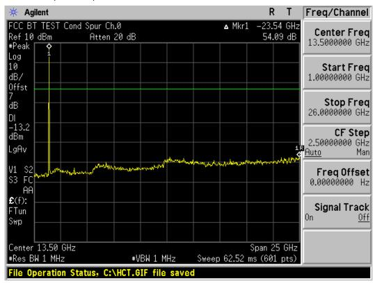
Test Plots (GFSK) - 1 GHz - 26 GHz (RBW:1 MHz, VBW: 1 MHz) Spurious Emission (Mid-CH)
