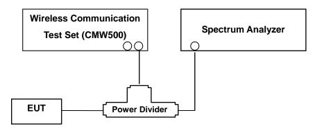
(Configuration of conducted Emission measurement) Test Procedure
