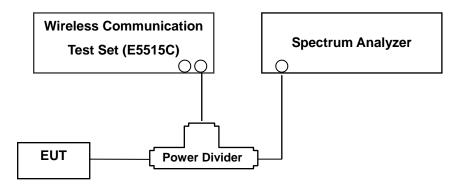
(Configuration of conducted Emission measurement) Test Procedure
