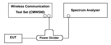
(Configuration of conducted Emission measurement) Test Procedure
