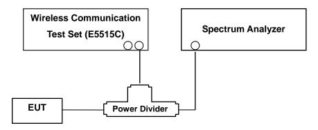
(Configuration of conducted Emission measurement)
