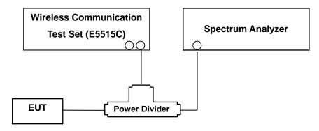
(Configuration of conducted Emission measurement) Test Procedure
