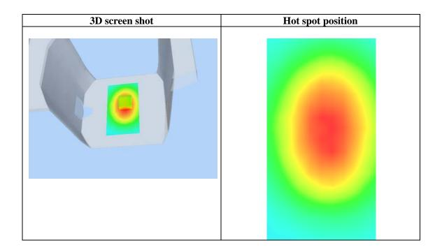
Test Laboratory: AGC Lab GSM 850 Middle-body- Worn-Back (MS) DUT:GSM MOBILE PHONE; Type:VZ102music
