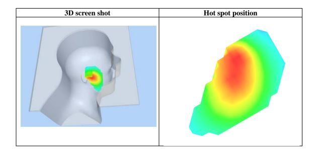
Test Laboratory: AGC Lab GSM 850 Mid-Body-Worn Front DUT:GSM MOBILE PHONE; Type:VZ102music
