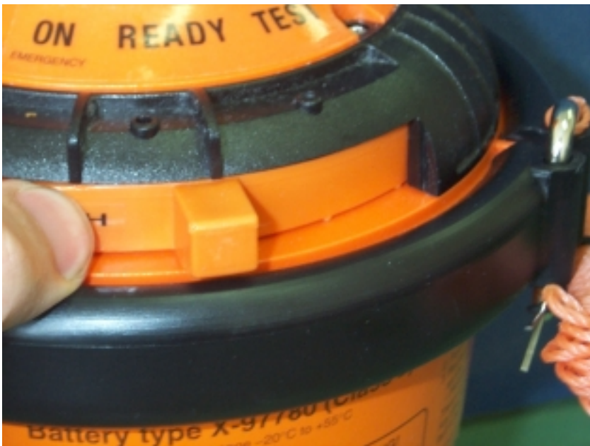
Photograph 4, shows thumb applying pressure to lever slide.
