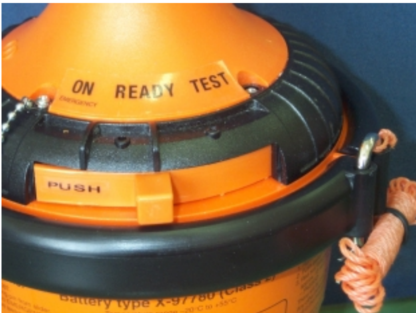
Photograph 2, first stage activation completed, note lever does not move.
