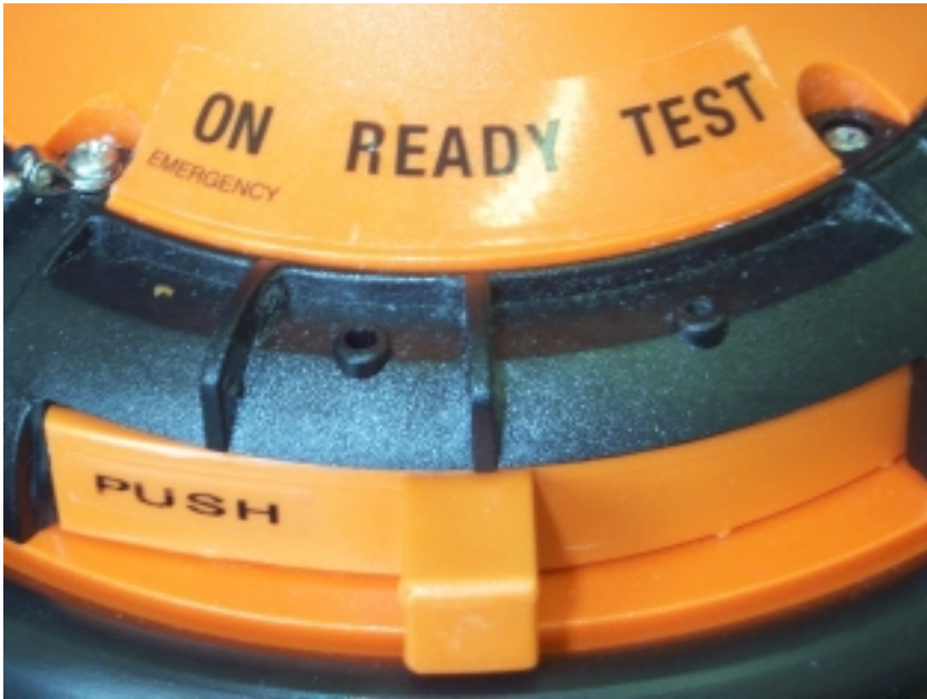
Photograph 3, shows lever slide, sprung section latched against black housing.
