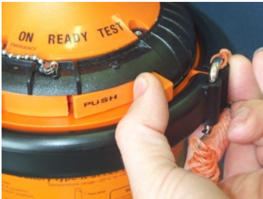
Photograph 6, shows lever slide in the "test" position.
