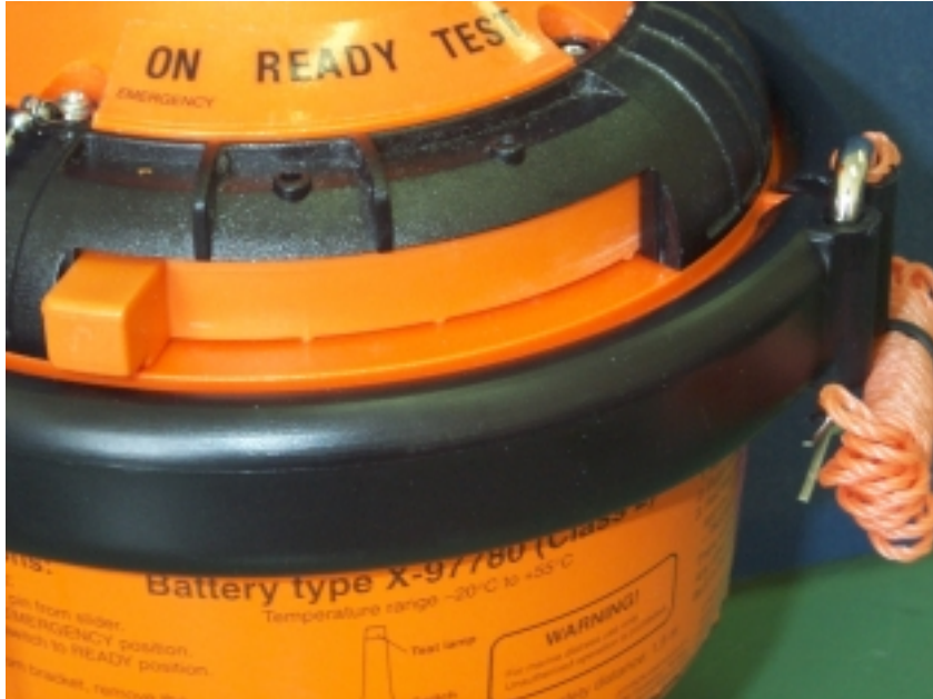
Photograph 5, shows lever slide in the "on" position.
