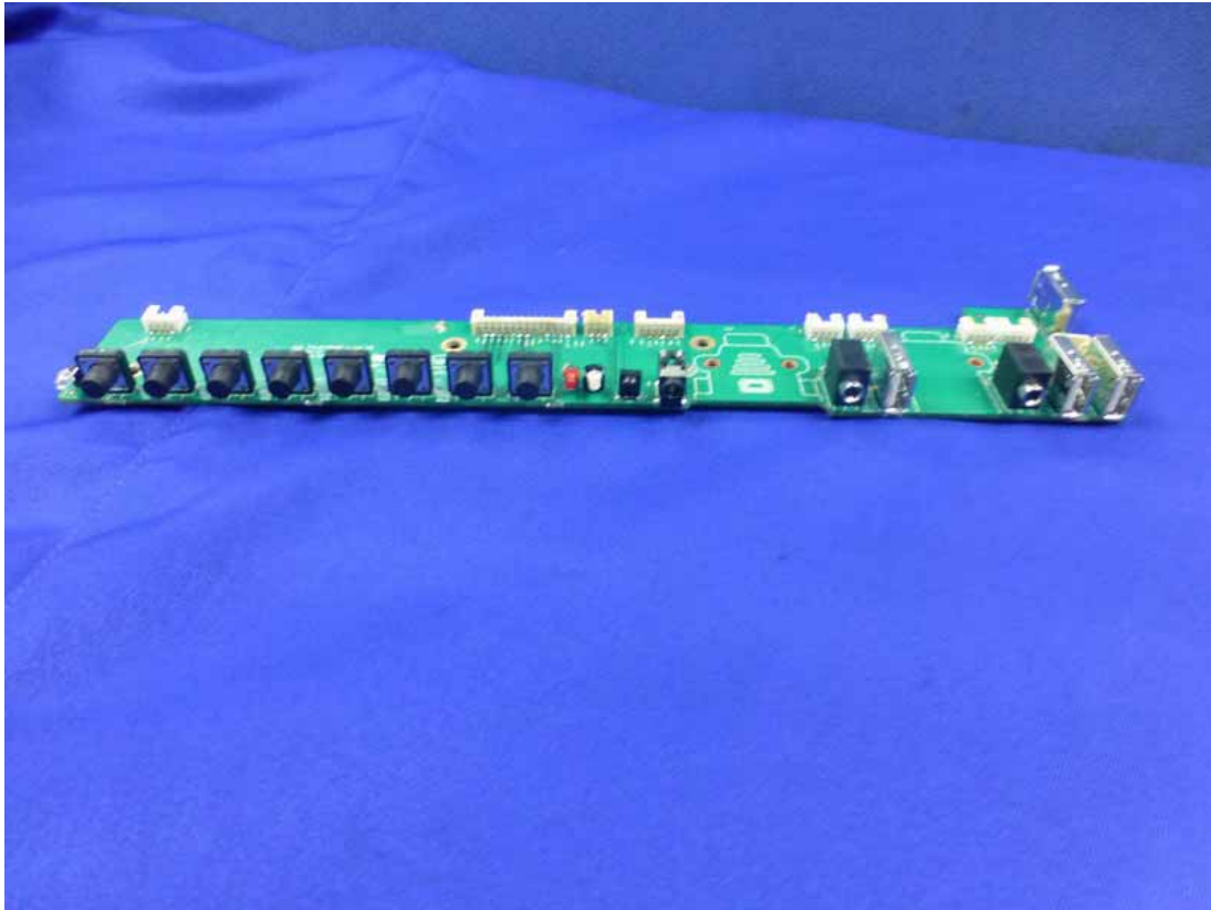
Figure 19 I/O Port of the Control Board
