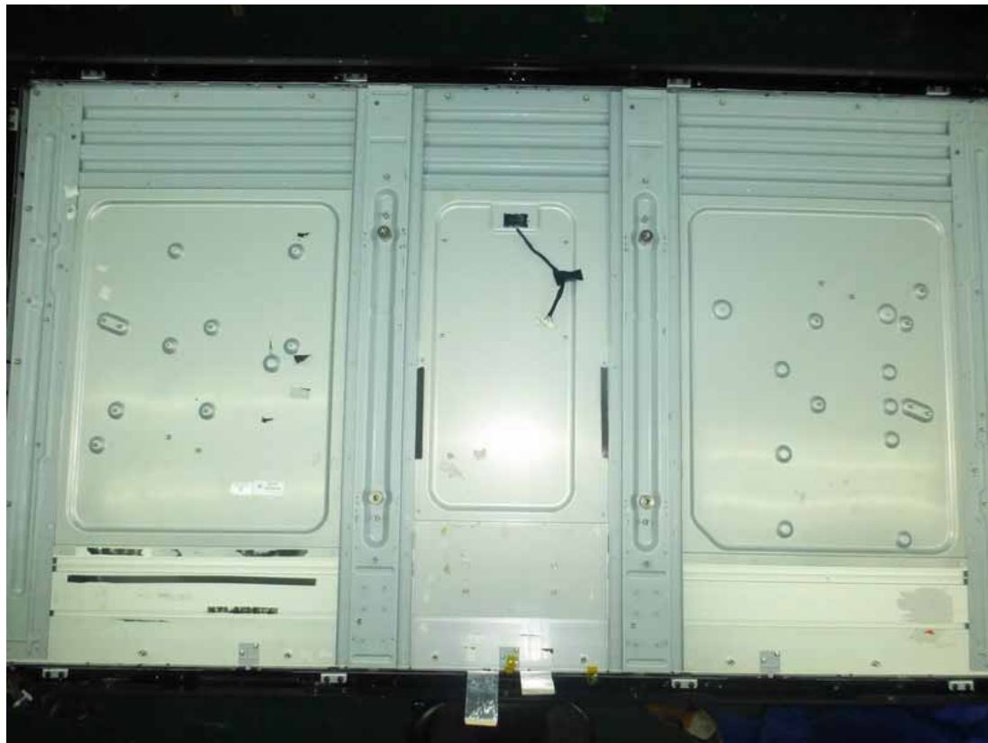
Figure 8 Backside of the LCD Panel
