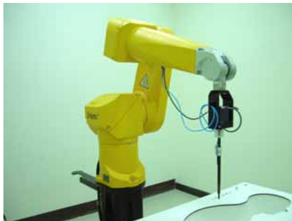
Fig. 5.2 Probe setup on robot
