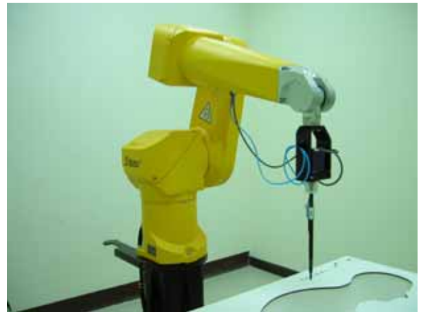
Fig. 5.2 Probe setup on robot
