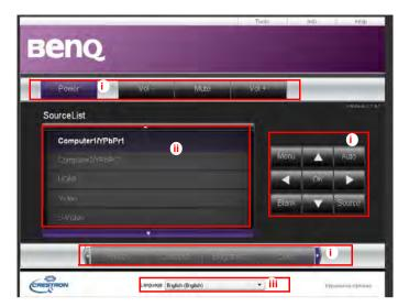
These buttons function the same as the ones on the OSD menus or remote control. See "2. PICTURE" on page 76 and "Remote control" on page 13 for details.
