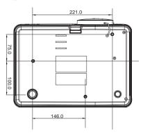
Ceiling mount screws: M4 x 8 (Max. L = 8 mm)
