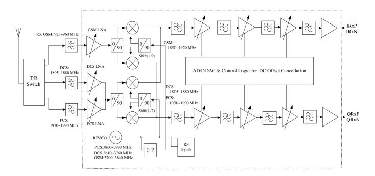
The Receiver structure in HD155155NP is a zero-IF solution. That means RF signal is directly down-converted to the baseband signal. And by the way, all of the DC-offset canceling processes are done within chip. We do not have to care about that.
