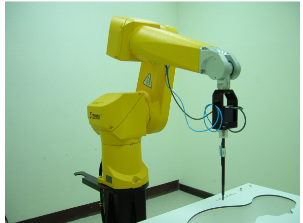
Fig. 5.2 Probe setup on robot
