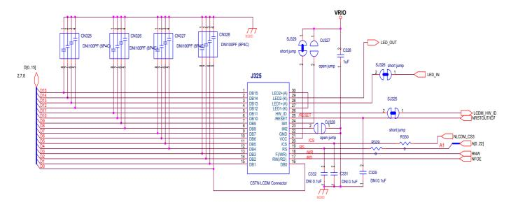
LCDM\_HW\_ID ( ADIN1 ) voltage allocation vs LCDM vendor : (we use the ADIN1 (Iota) to detect the LCDM vendor)
