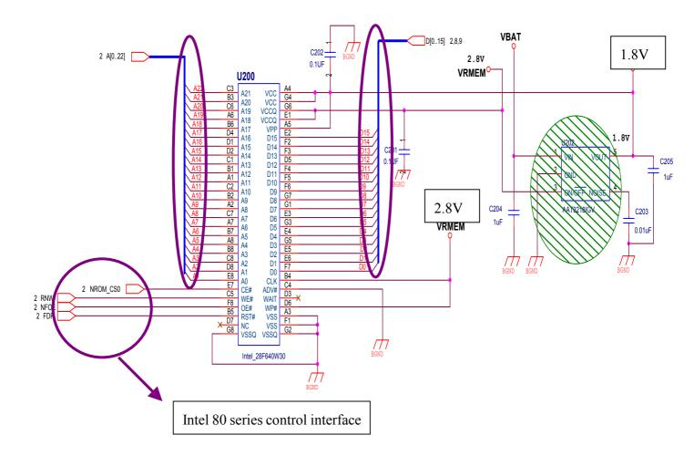
Above schematic is the Flash , below is the 1-T SRAM schematic
