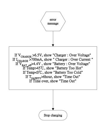
error 0 : "Illegal Battery" error 1 : "Charger : Over Voltage" error 2 : "Charger : Over Current " error 3 : "Battery : Over Voltage" error 4 : "Battery Too Hot" error 5 : "Battery Too Cold" error 6 : "Time Out"
