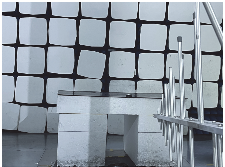
Radiation Emission Test Setup (30MHz to 1GHz)
