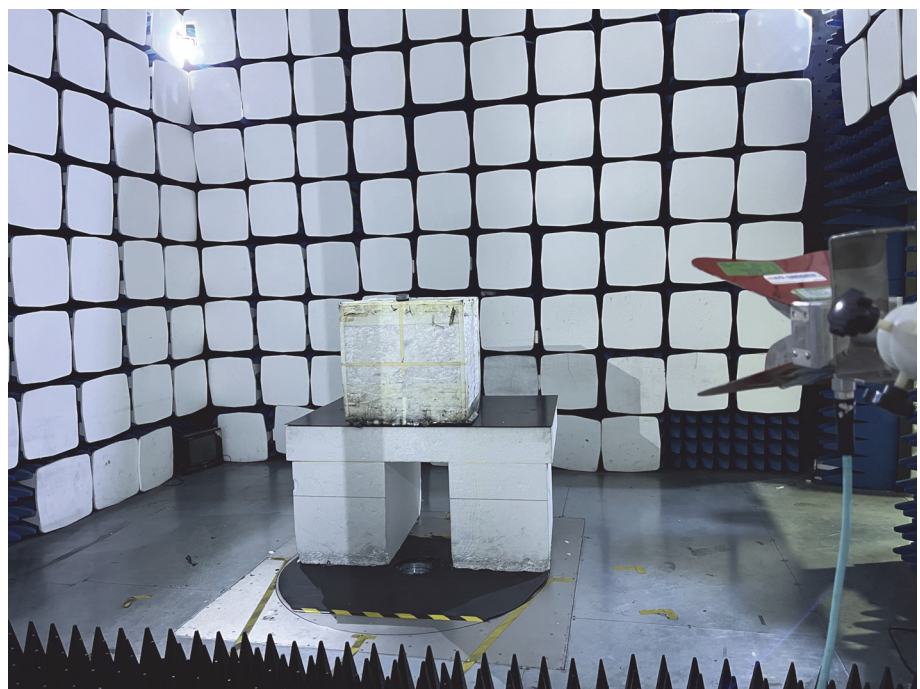
Radiation Emission Test Setup (1GHz to 18GHz)
