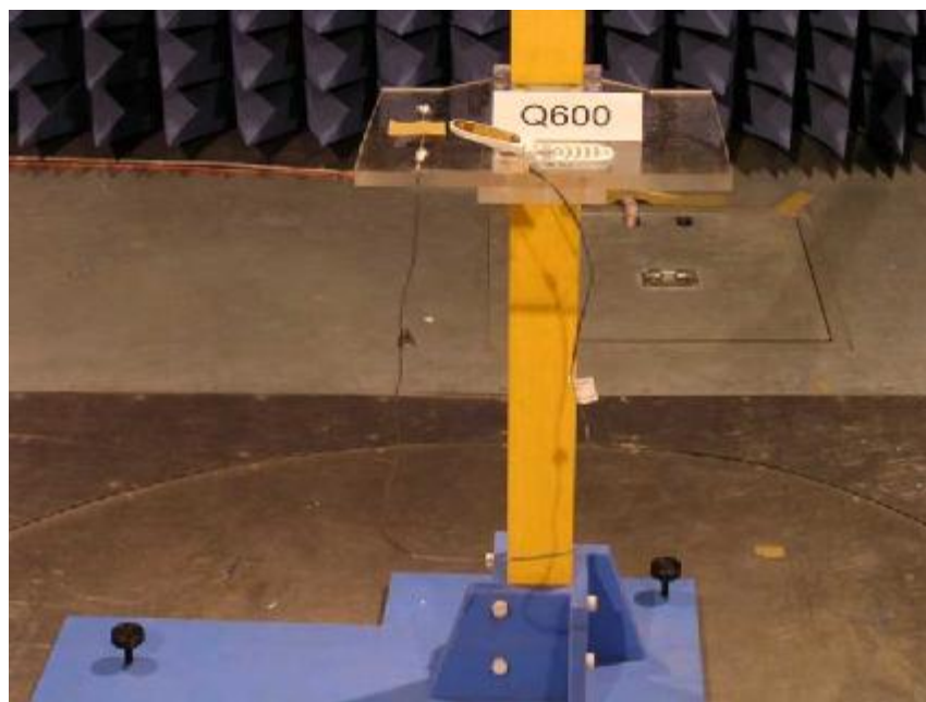
Photo 1: Radiated Spurious set-up photo
