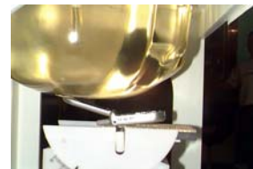
Figure 14.2 Right Head SAR Test Setup -- Ear / 15° Tilt Position --
