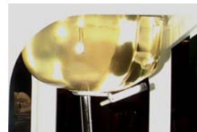
Figure 14.1 Right Head SAR Test Setup -- Cheek / Touch Position --
