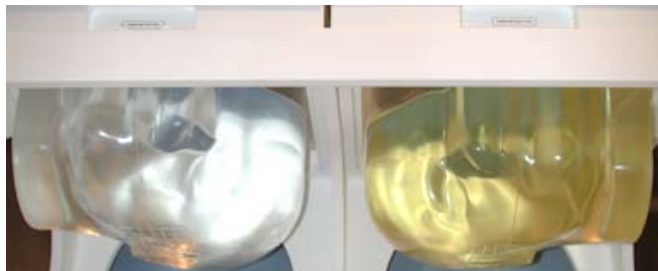
Figure 7.1 Left and Right SAM Phantom shells
