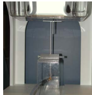
Figure 12.1 Dipole Validation Test Setup
