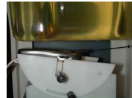
Figure 14.5 Body SAR Test Setup -- w/o Holster --
