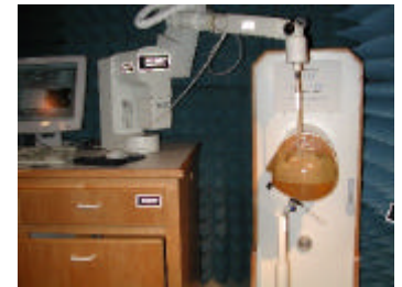
Fig. 1 SAR Test Setup
