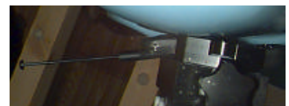
Figure 18. PCS CDMA Head SAR Test Setup
