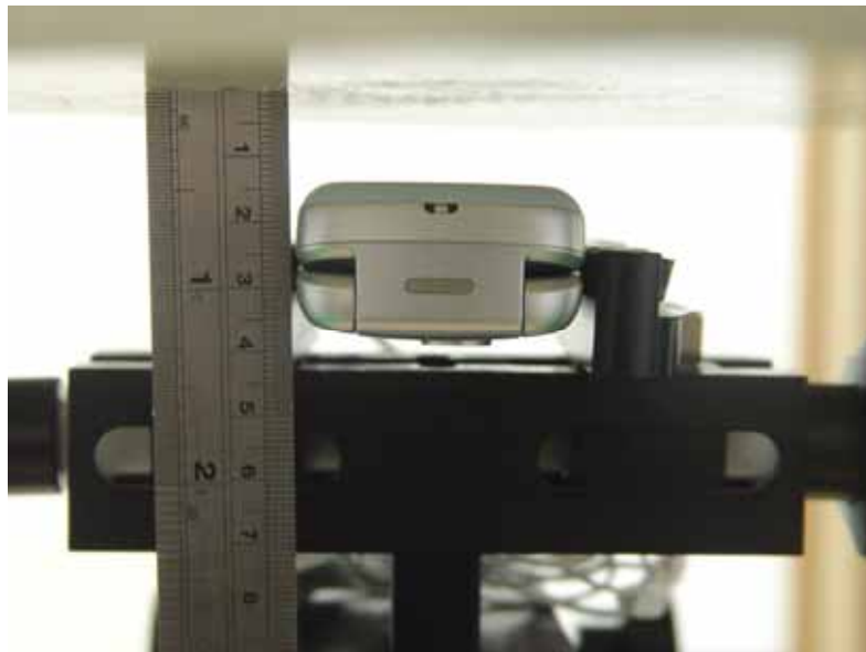
Fig. 9.8 Keypad Down with 1.5cm Gap
