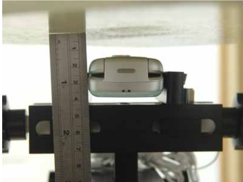
Fig. 9.7 Keypad Up with 1.5cm Gap
