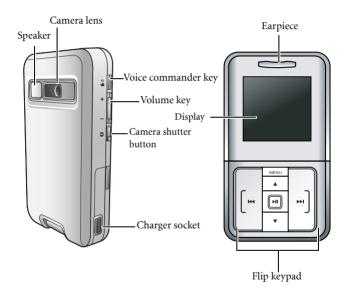
The flip keypad is used for performing the MP3 function and for answering and ending a phone call.
