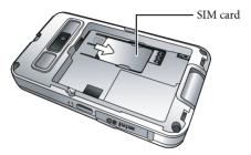
If you wish to remove the SIM card, first press down the locking tab, then slide the SIM card out in the direction of the arrow as illustrated.
