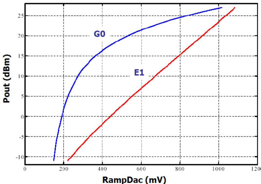
In E1 mode, Vramp controls the RF output signal in a LIN-LOG characteristic meaning that the RF output power expressed in [V].
