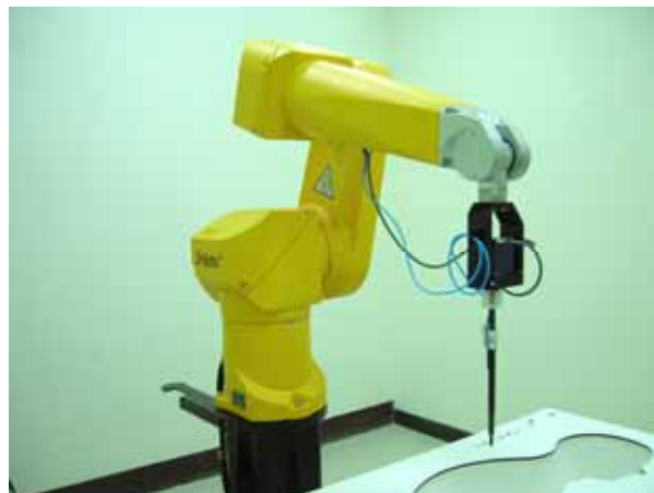
Fig. 5.2 Probe setup on robot
