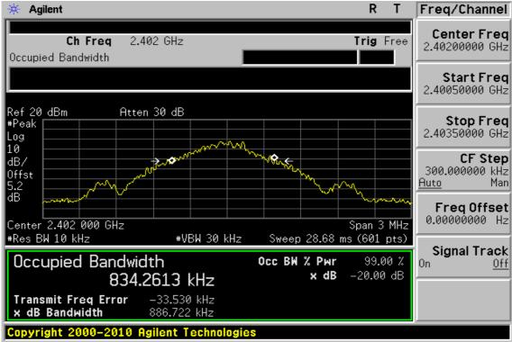
20dB Bandwidth Test Data CH-Mid
