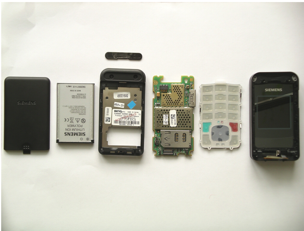
AF51 disassembly step1 (base, left)
