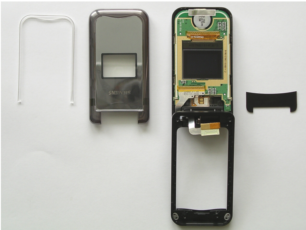
AF51 disassembly step2 (flip, left)
