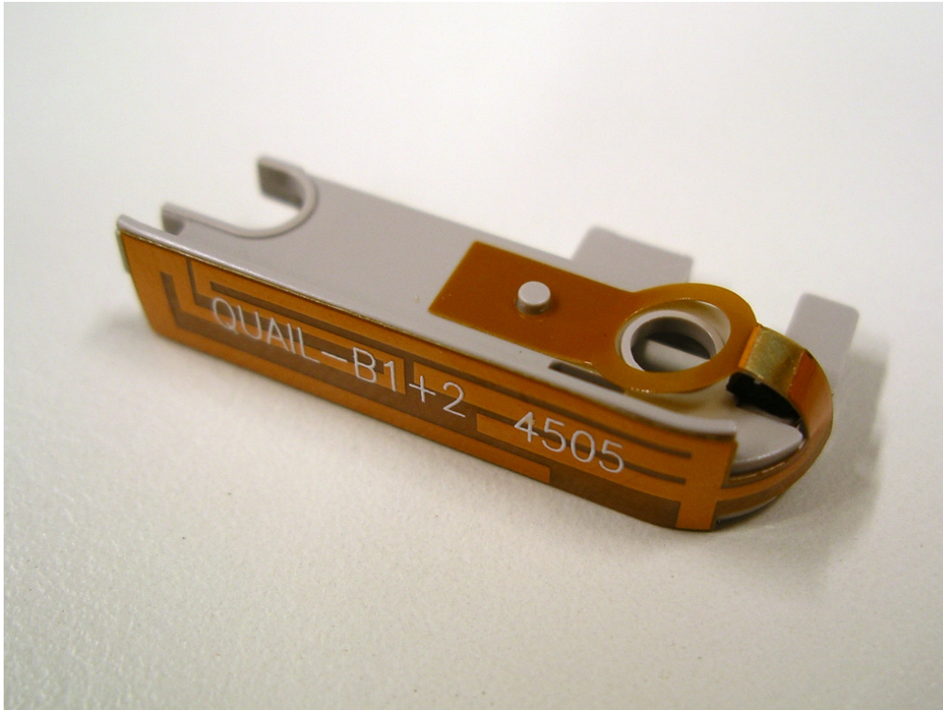
AF51 tri-band antenna
