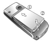
Switch off your phone before removing the battery.
