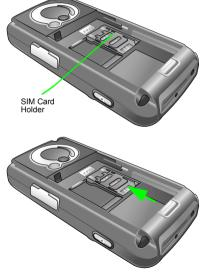
2. Push the SIM card holder in the direction of the arrow (as shown in the figure to the right) to unlock it.
