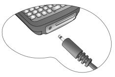
2. Disconnect the charger cable when charging completes.
