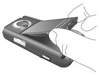
2. With the top half in position, push down the remaining battery into the compartment. The battery latch will click to secure the battery in place.
