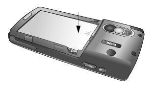
4. Push the battery door down on the phone and slide it into place.
