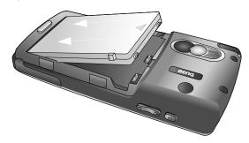
3. Push the battery against the top of P31 to insert the teeth into the holes, then press the battery down gently to click it back into place.
