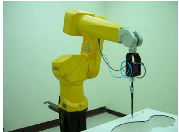
Fig. 5.2 Probe setup on robot
