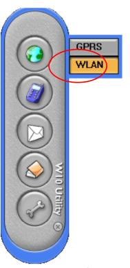
When users choose network configuration, the submenu will pop up. Left click the mouse on the WLAN item and the WLAN control panel will pop up.
