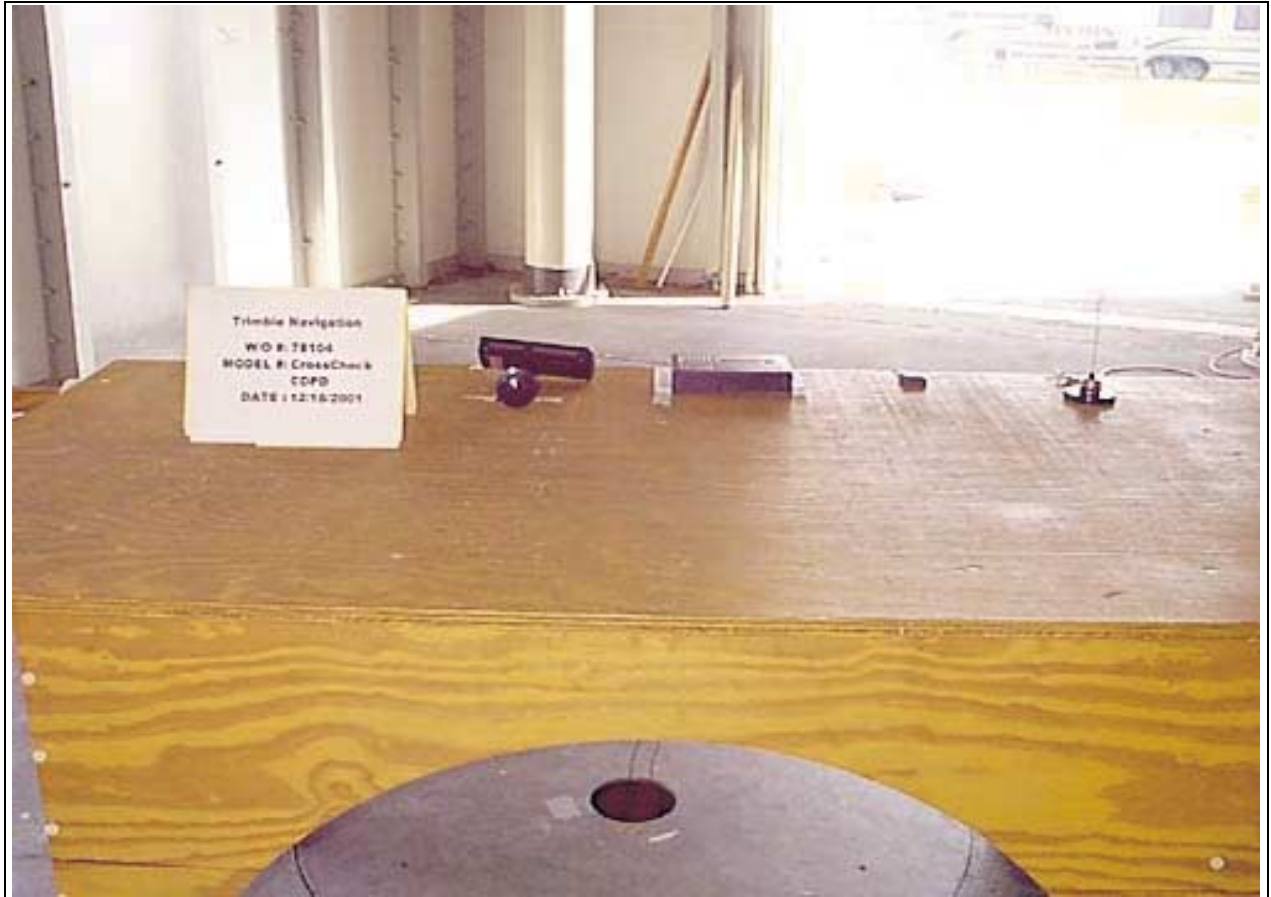
Radiated Emissions - Front View
