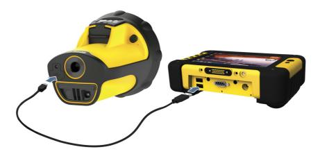
Once connected, use the GNSS field software to configure the connection (see below).
