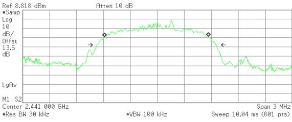
Occupied Bandwidth 1.1493 MHz Occ BW % Pwr 99.00 % x dB -26.00 dB
