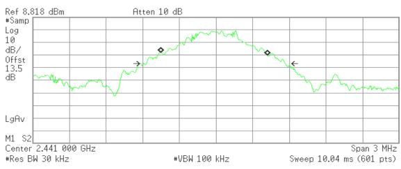
Occupied Bandwidth 869.8414 kHz Occ BW % Pwr 99.00 % x dB -26.00 dB
