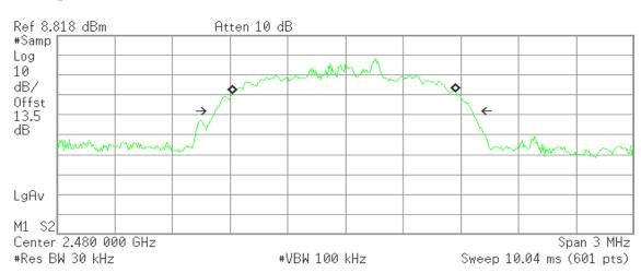
Occupied Bandwidth 1.1572 MHz Occ BW % Pwr 99.00 % **x dB** -26.00 dB
