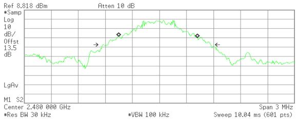
Occupied Bandwidth 867.4311 kHz Occ BW % Pwr 99.00 % x dB -26.00 dB
