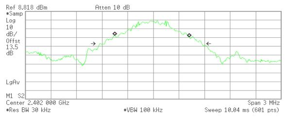
Occupied Bandwidth 870.4522 kHz Occ BW % Pwr 99.00 % x dB -26.00 dB
