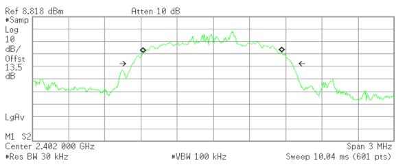
Occupied Bandwidth 1.1476 MHz Occ BW % Pwr 99.00 % x dB -26.00 dB
