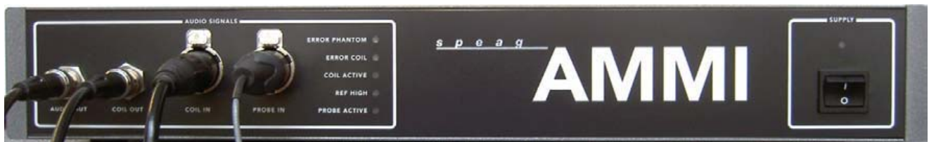
Figure 4.4: AMMI front panel
