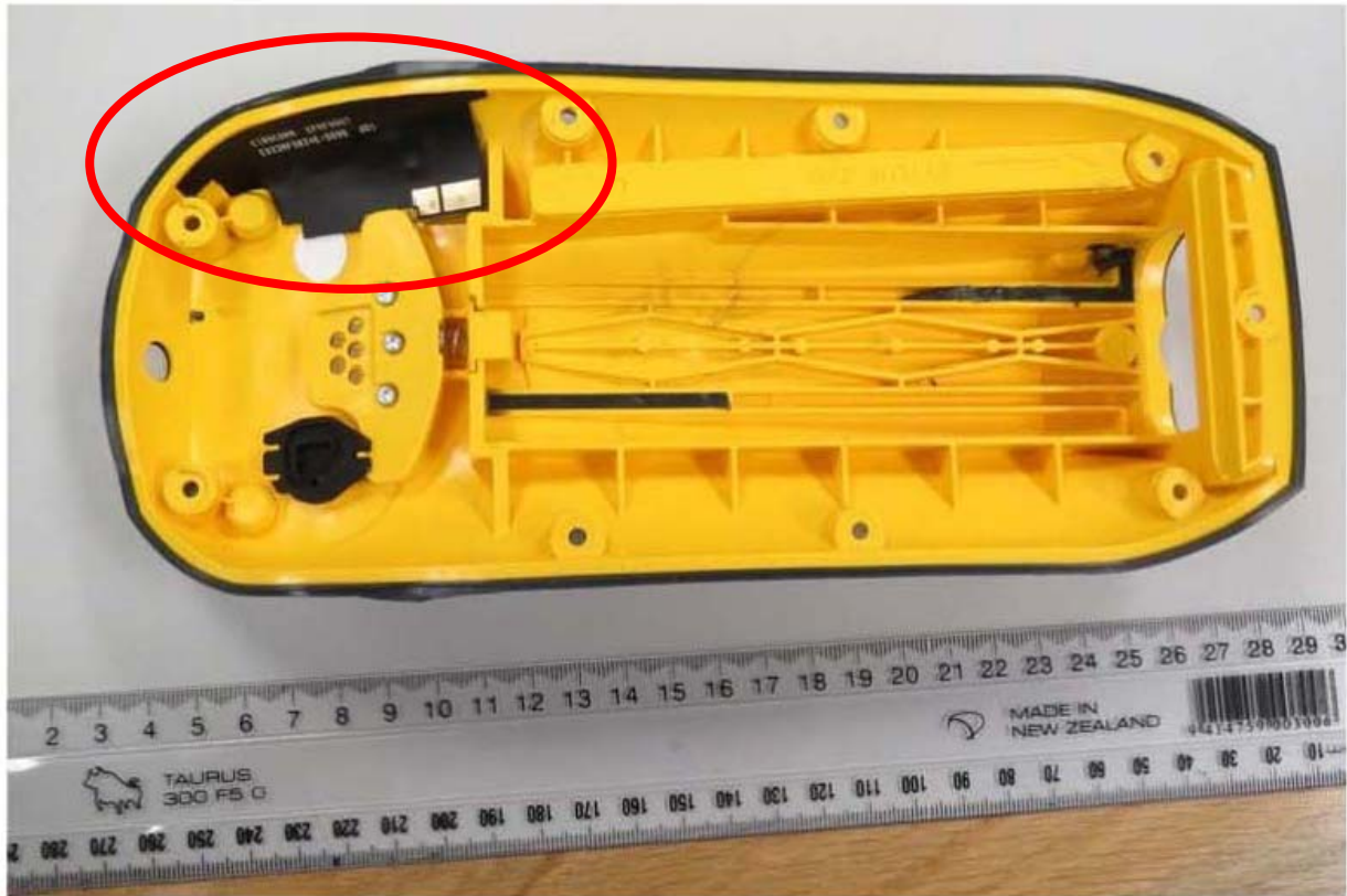
Lower half of enclosure showing Cellular Antenna
