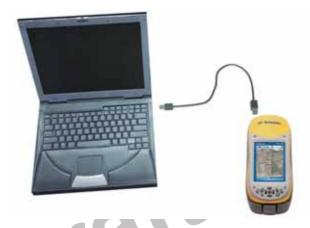
Connecting the handheld to a computer using the USB data cable Figure 4.1
