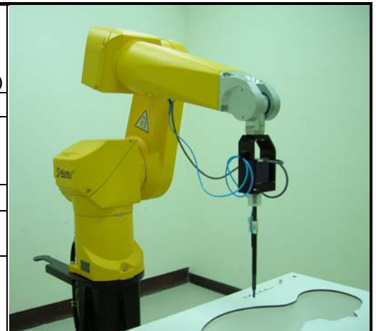
Fig. 5.2 Probe Setup on Robot
