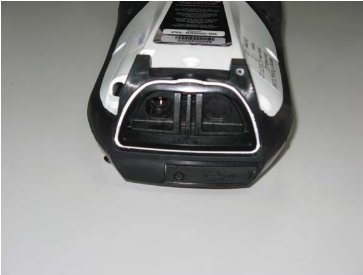
Fig 3 Rear End view showing replaceable Battery
