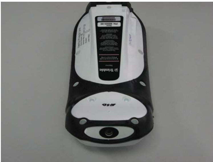
Fig 2 Front End View showing Camera Lens
