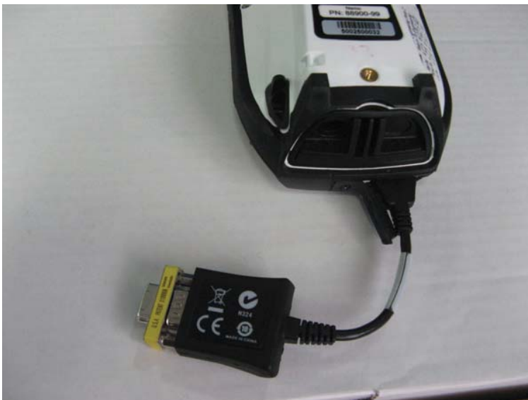
Fig4 Rear End view showing Serial adapter accessory connection
