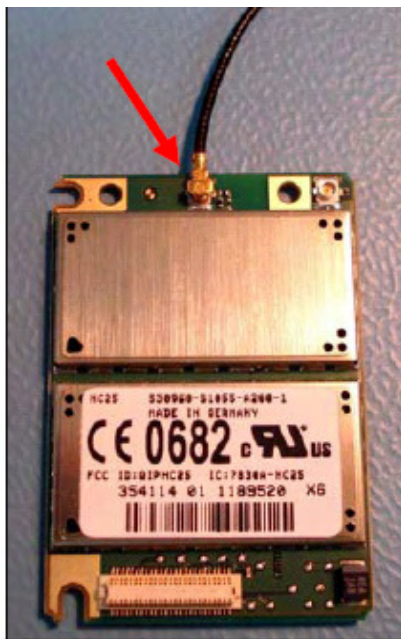
Fig2 Close up of HC25 Modem Card—GeoExplorer XH 3.5G and XT 3.5G only
