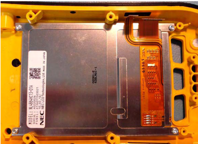
Fig 5 Rear view of Display/Touch screen
