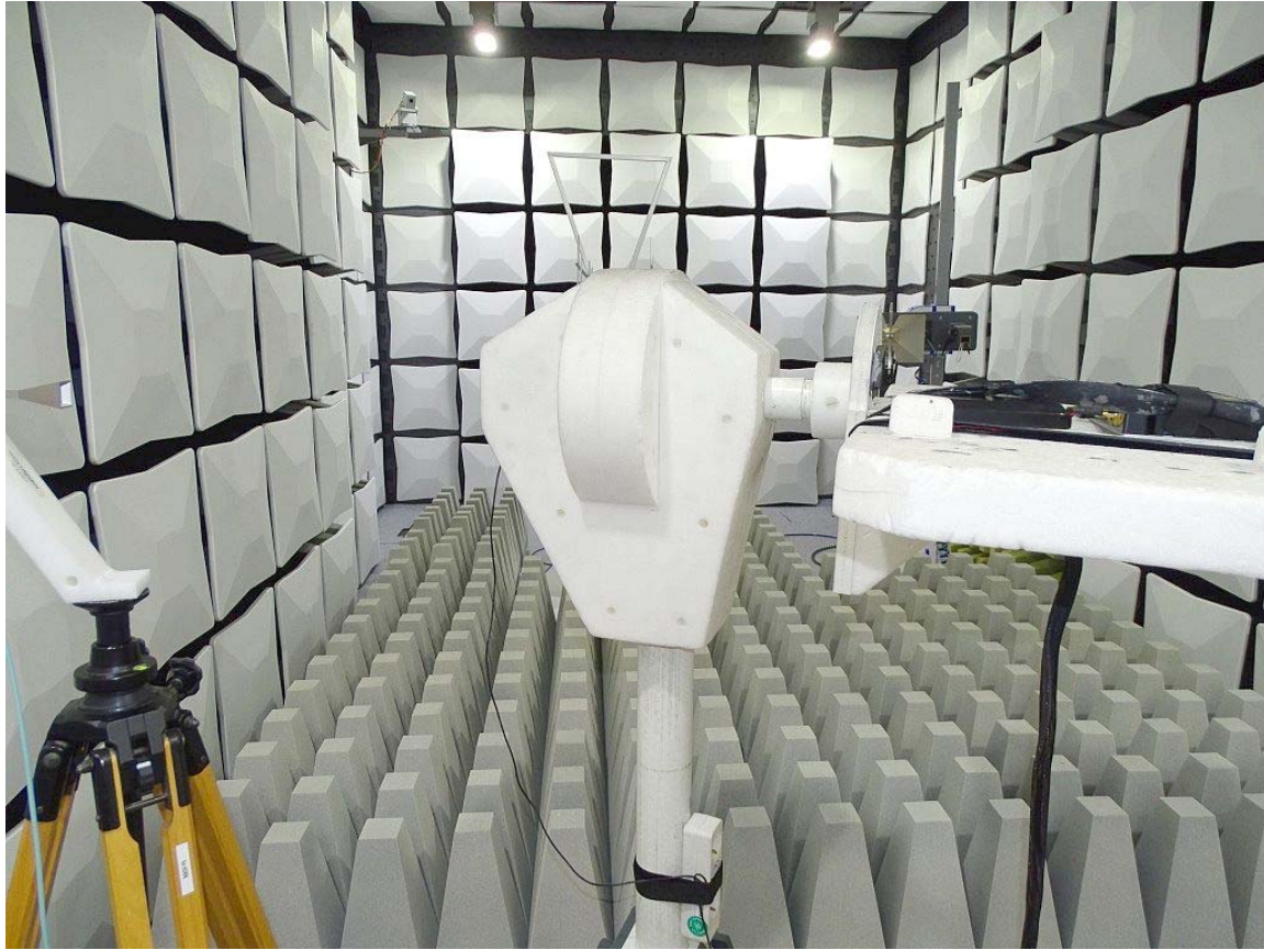
Photo 4: Test setup for radiated measurements (Enclosure, fully-anechoic chamber, 26-40 GHz intentional radiator §15, ANSI C63.10)
