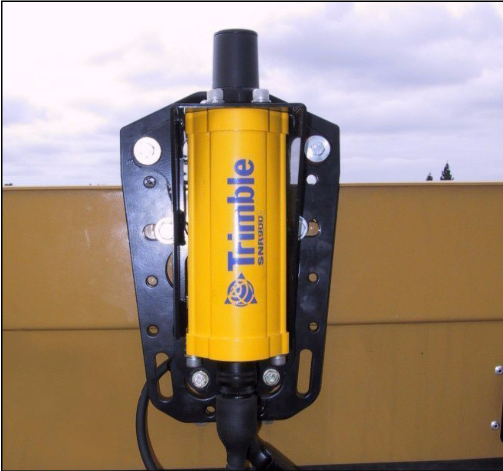
Figure 4.4 SNR900 mounted at the rear of a cab roof
