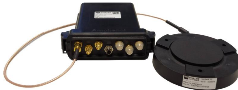
RFID Reader/Writer with connected antenna (No. :SMSE015)
