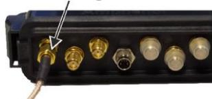
2. Connect the second antenna to the second connection of the RFID Reader/Writer. Proceed in the same way as for the first antenna.
